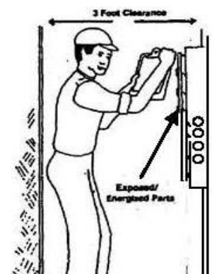
Wall not grounded. e.g. Plasterboard on Wood Studs
